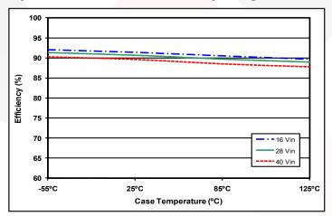
Figure 5: Efficiency at 60% load (2.4A load on +15V and 2.4A load on -15V) versus case temperature for Vin = 16V, 28V, and 40V.
