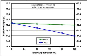
Figure 10: Load regulation vs. total output power from zero to to full load where -Iout equals three times +Iout at nominal input voltage and TCASE  $= 25^{\circ}C.$
