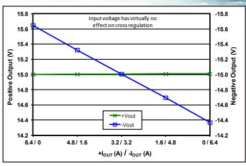
Figure 8: Load regulation vs. load current with power fixed at 80% load (96W) and load currents split as shown between the +15V and -15V outputs, at nominal input voltage and TCASE = 25°C.
