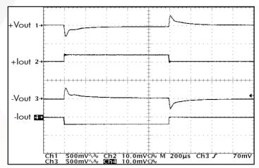
Figure 18: Output voltage response to step-change in total load current (0%-50%-0%) of total lout (max) split 50%/50%. Load cap:  $1\mu F$  ceramic cap and  $10\mu F$ , 100 m $\Omega$  ESR tantalum cap. Ch 1: +Vout (500 mV/div); Ch 2: +Iout (5A/div); Ch 4: -Vout (500 mV/div); Ch 4: -Iout (5A/div).
