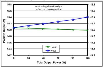
Figure 9: Load regulation vs. total output power from zero to to full load where +Iout equals three times -Iout at nominal input voltage and TCASE  $= 25^{\circ}C.$
