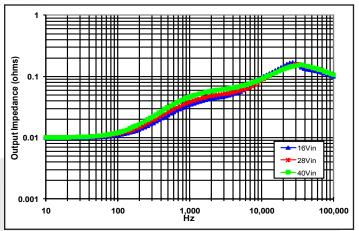
Figure 25: Magnitude of incremental output impedance ( $+Z_{out} = +v_{out}/+i_{out}$ ) for minimum, nominal, and maximum input voltage at
