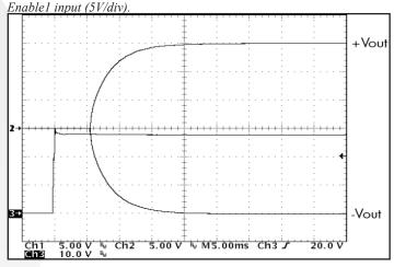
Figure 16: Turn-on transient at full load, after application of input voltage (ENA 1 and ENA 2 logic high) (5 ms/div). Ch 1: +Vout (5V/div); Ch 2: -Vout (5/div); Ch 3: Vin (10V/div).
