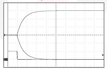
Figure 23: Rise of outpit voltage after the removal of a short circuit across the positive output terminals. Ch 1: +Vout (5V/div); Ch 2: -Vout (5/div); Ch 3: +Iout (10A/div).
