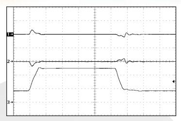
Figure 19: Output voltage response to step-change in input voltage (16V - 50V - 16V). Load cap: 10µF, 100 m□ ESR tantalum cap and 1µF ceramic cap. Ch 1: +Vout (500mV/div); Ch 2: -Vout (500mV/div); Ch 3: Vin (20V/div).
