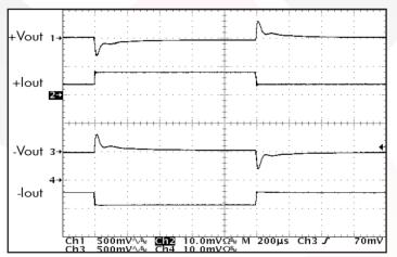
Figure 17: Output voltage response to step-change in total load current (50%-100%-50%) of total lout (max) split 50%/50%. Load cap:  $1\mu$ F ceramic cap and  $10\mu$ F,  $100\ m$  $\square$  ESR tantalum cap. Ch 1: +Vout (500 mV/div); Ch 2: +Iout (5A/div); Ch 3: -Vout (500 mV/div); Ch 4: -Iout (5A/div).
